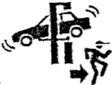
( 10 ) Position Vehicle with center of gravity midway between adapters. .
